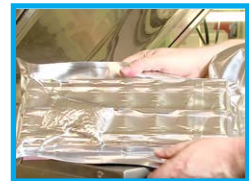
The devices are then re-baked & vacuum packed with MSL desiccant
