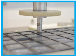
Automated vacuum pickup arm transports the device from the tray
