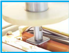
The device is fluxed, each side in sequence
