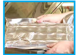
The devices are cleaned, then re-baked & vacuum packed with MSL desiccant
