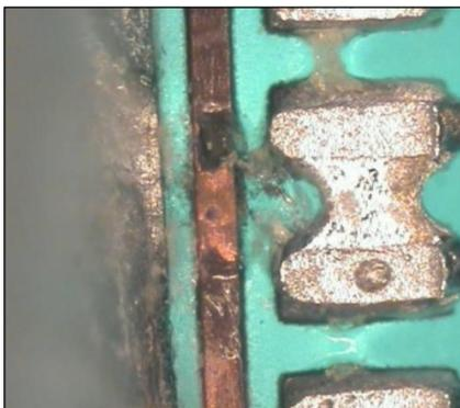
**Flux residues with potential to cause shorts & current leakage**
