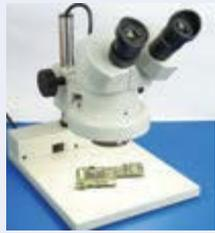
Visual inspection criteria employed by Retronix conforms to IDEA-STD-1010-B, MIL-STD-883G and the mechanical dimension criteria of product datasheets. These tests will not only find remarked devices, they will also be able to tell if the components are NEW and UNUSED.
