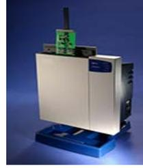
Ionic test is performed to measure the level of ionic residues which is a good indicator of the cleanliness of the IC. Retronix provide a full report that details the sample size, contamination value & device type.
