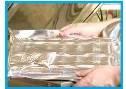
The devices are then cleaned, re-baked & vacuum packed with MSL/Dessicant
